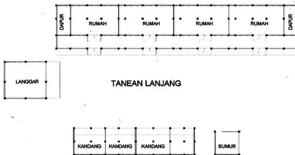
**Figure 9.** Tanean Length Layout Model, in Torjun District, Sampang Regency, Madura, Has a North-South Building Direction
